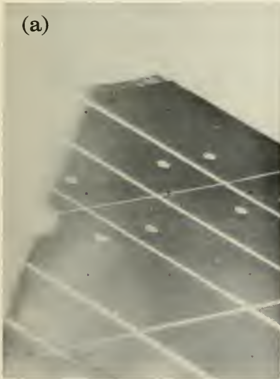
FIGURE 4-31.—Top of Surveyor V compartment B. A clump of soil ejected onto the compartment top during the firing splattered in a direction away from vernier engine 1. (a) Pre-firing picture (Sept. 10, 1967, 02:29:29 GMT). (b) Postfiring picture (Sept. 20, 1967, 05:48:58 GMT).
