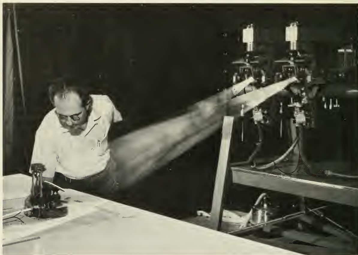
FIGURE 3-14.—Surveyor photorestitutor. This instrument was originally designed to rectify monoscopic Surveyor pictures, but has been modified for use as an anaglyphic stereoplotter. Each projector is a geometric analog of the television camera. Glass transparencies, or "diapositives," made from stereoscopic pairs of pictures are used at each camera position. The projectors and projector mirrors are set in the same relative orientations as the camera at the time each picture was taken. One picture is projected with red light; the other is projected with blue light onto a white screen, or platen. The operator wears spectacles with one red lens and one blue lens, enabling him to see the overlapping images as a single three-dimensional picture or model. As the platen is moved vertically or horizontally, the point of light at its center appears to float in the stereoscopic model. The horizontal position of the point of light is plotted on the map manuscript over which the platen carriage, or tracing table, moves. The vertical position of the point of light can be read from a counter on the tracing table.
