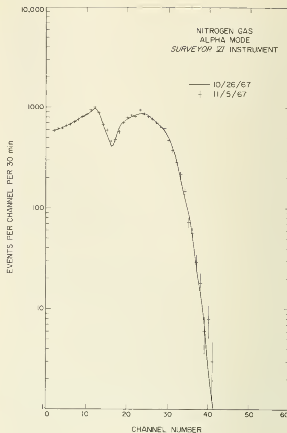
FIGURE 8-19.—Alpha-scattering spectra of nitrogen gas taken during prelaunch tests of the Surveyor VI instrument.
