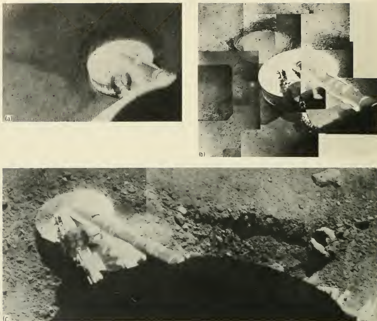
FIGURE 4-6.—Lunar surface areas disturbed during footpad 2 landing impacts. (a) Surveyor I: wide-angle picture showing rayed ejecta pattern (June 5, 1966, 11:29:49 GMT). (b) Surveyor III: mosaic showing high reflectivity of bottom of first two overlapping imprints outboard of footpad. Edge of a third imprint, formed in ejecta from first two impacts, is visible over top of footpad (Apr. 26, 1967, Catalog 3-MP-3). (c) Surveyor V: wide-angle pictures showing trench formed as spacecraft slid down the inner slope of the small crater in which it landed. The deepest penetration was on the uphill end of the trench where initial impact occurred (Sept. 14, 1967, Catalog 5-MP-19). (d) Surveyor VI: after initial landing. Wide-angle frames showing part of imprint made during first impact and symmetrically distributed ejecta formed when the spacecraft had a near-vertical final descent onto an almost horizontal lunar surface (Nov. 15, 1967, Catalog 6-SE-25). (e) Surveyor VI: after hop. Part of mosaic of wide-angle pictures showing portion of imprint made during first impact at right of footpad: spacecraft bounded back toward prehop position after making this imprint. Most soil was ejected in the direction the spacecraft was moving during the hop (Nov. 17, 1967, Catalog 6-SE-9). (f) Surveyor VII: imprint made during first impact is to the lower right of the footpad. The rock beside the footpad is about 20 cm across (Jan. 14, 1968, Catalog 7-SE-18).
