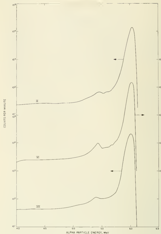
FIGURE 8-14.—Composite energy spectra for each of the three sets (six sources each) of the curium-252 flight sources.
