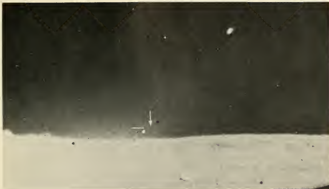
FIGURE B-5.—View of the sunset position taken over 14 hours after sunset by the Surveyor VII television camera. This wide-angle picture, made in the integration mode of the camera, shows the faint, residual solar corona and the lunar surface illuminated by earthlight. The bright spot in the sky is Mercury, spread by the camera's white spread function and elongated by lunar rotation during the 30-minute exposure time (Jan. 23, 1968, 20:45:55 GMT).
