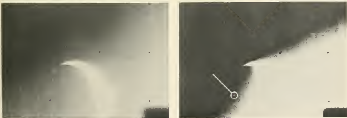
FIGURE 11-3.—A comparison of these two pictures clearly reveals the Tucson laser beam. The picture was digitized by the JPL Image Processing Laboratory, and the contrast then "stretched." (a) Jan. 19, 1968, 08:41:53 GMT. (b) Portion of the digitized, stretched picture; the spot produced by the laser is indicated.
