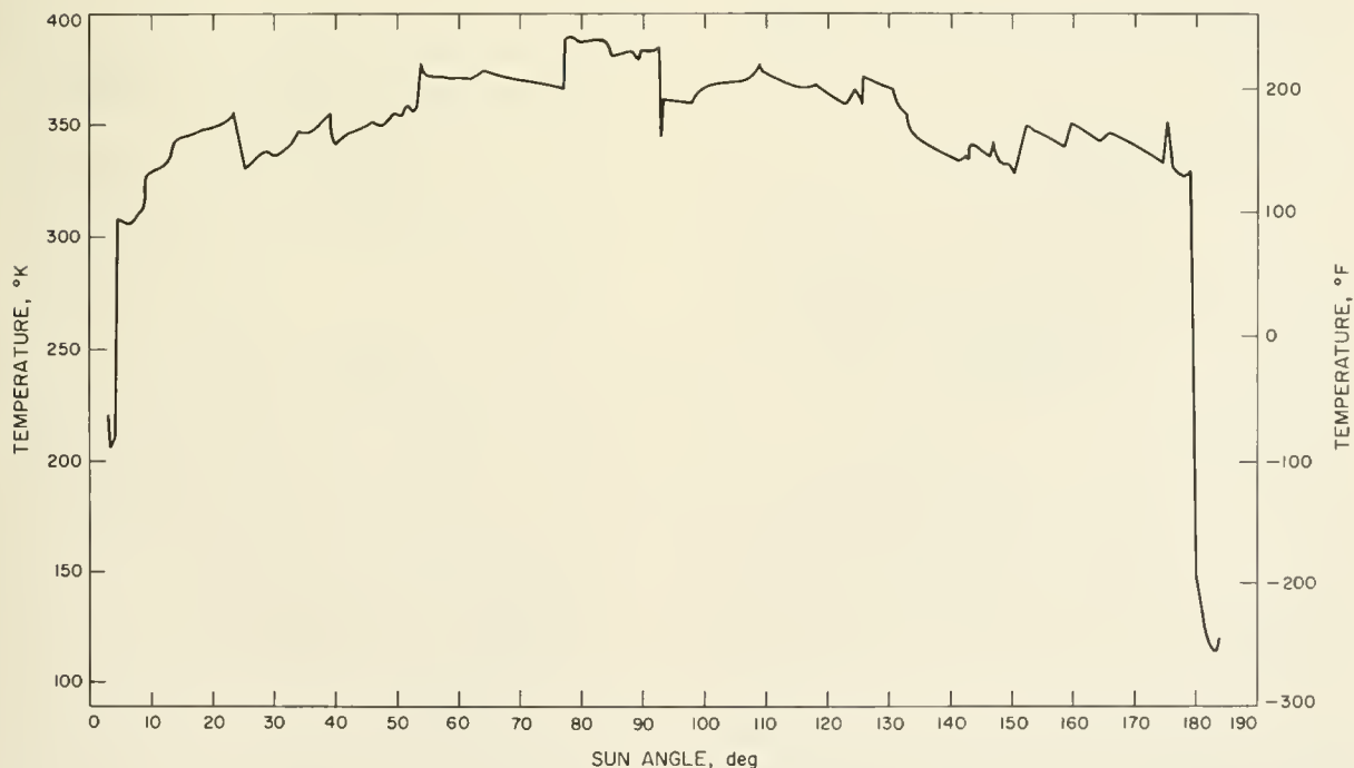
FIGURE 6-26.—Temperature of Surveyor VI solar panel.
