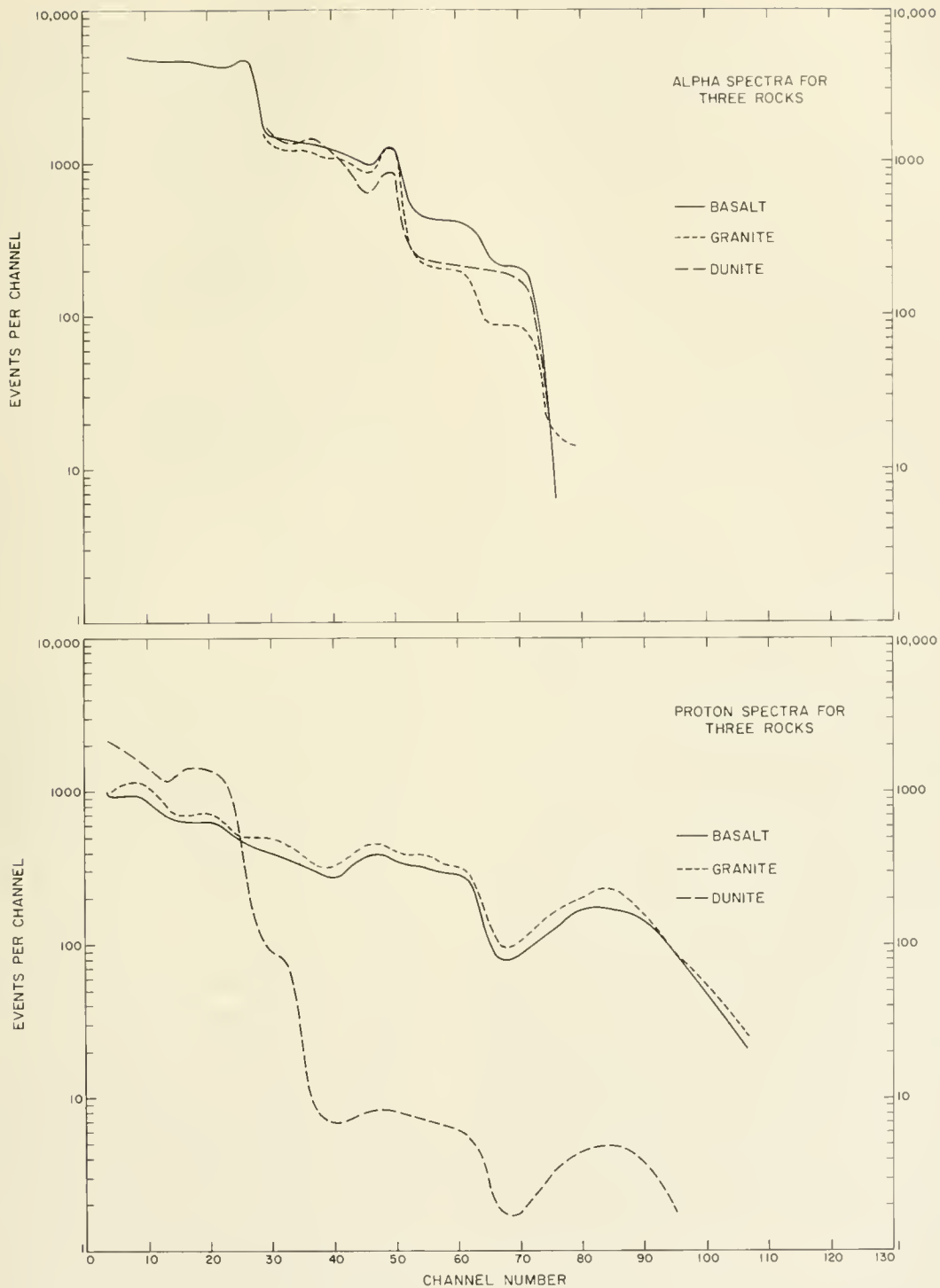
FIGURE 8-40.—Alpha-scattering instrument response from three rocks. Data taken with a Surveyor prototype instrument (P-2) on samples of basalt (USGS-W-1), granite (USGS-G-2), and dunite (USGS-DTS-1). All data from each rock have been multiplied by a factor to make the responses equal in the oxygen region of the alpha mode.
