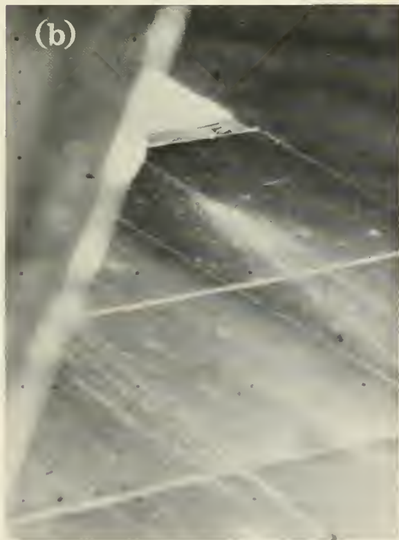
FIGURE 4-31.—Top of Surveyor V compartment B. A clump of soil ejected onto the compartment top during the firing splattered in a direction away from vernier engine 1. (a) Pre-firing picture (Sept. 10, 1967, 02:29:29 GMT). (b) Postfiring picture (Sept. 20, 1967, 05:48:58 GMT).
