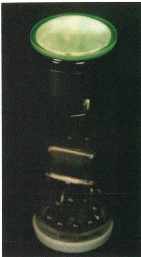
FIGURE 6. LAMPS WITH NANOTUBE field emitters. This lighting element has a field-emitting cathode that consists of a film of nanotubes. Different colors can be produced using different fluorescent elements on the phosphor display screen. (Adapted from ref. 14.)
