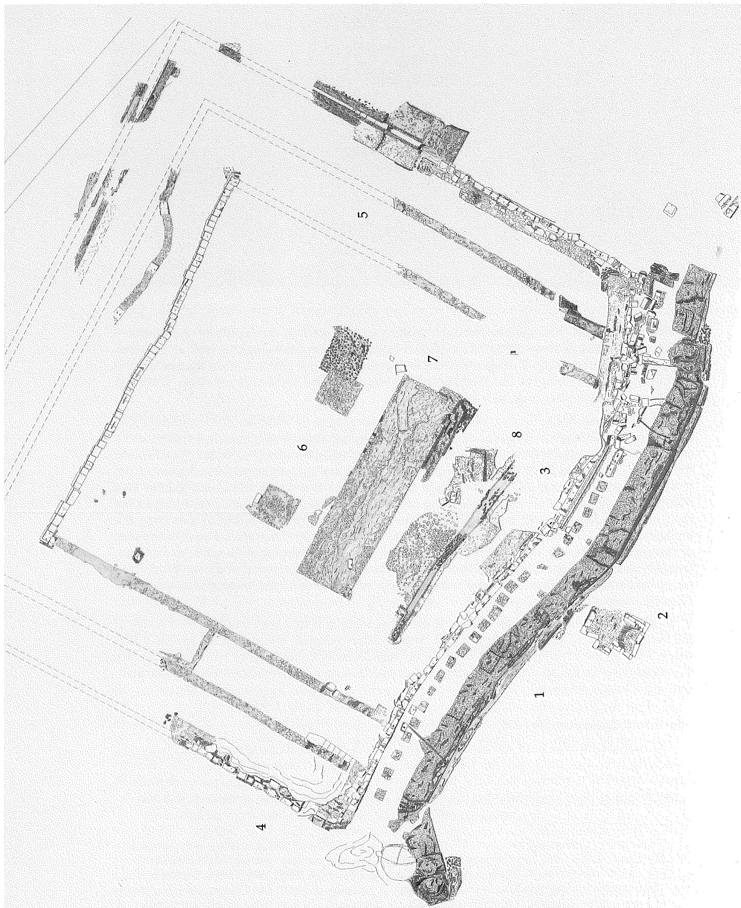
Fig. 4. Octavian's tropaeum , present state. Lower terrace: 1. The first retaining wall. 2. Ruins of naiskos. 3. Second retaining podium wall. 4. W and E sides of the platform. Upper terrace: 5. Stoa. 6. Pedestals. 7. Monumental altar. 8. Pipe for drainage.
