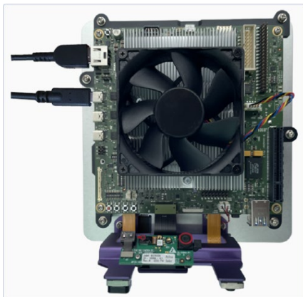
Figure 4-2 Connecting the IQ-X board to the host computer
