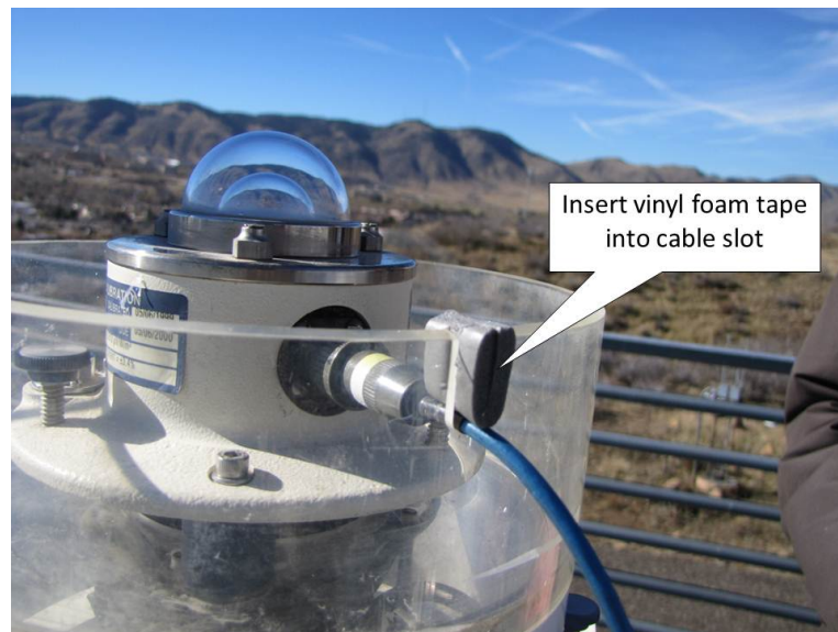
Figure 23. Plugging the slot with foam.
