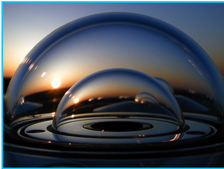
Figure 17. Two Schott Glass hemispheres protect the thermopile detector from the weather.
