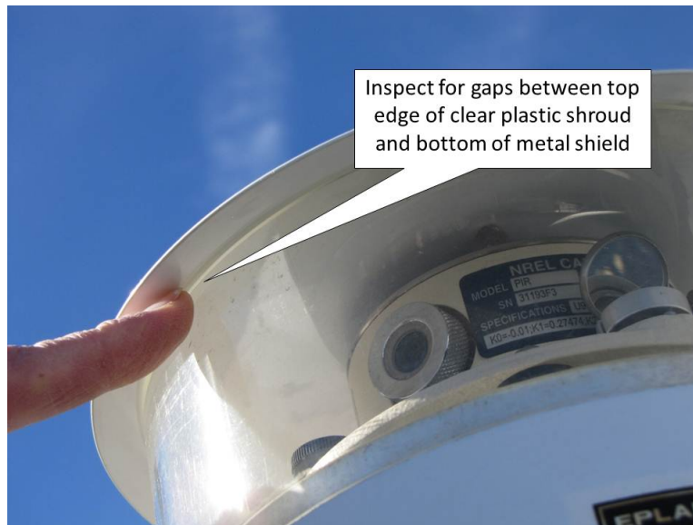
Figure 24. Inspecting for gaps under the sun shield.
