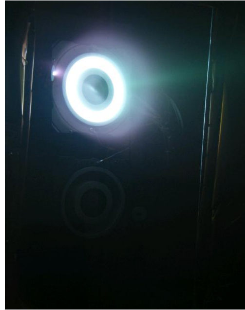
Figure 16. Nominal firing on first TMA-NG demonstrator. (2011 in LIA Snecma vacuum test bench) First cathode cross firing foreseen 3 rd quarter 2011
