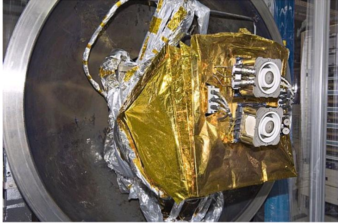
Figure 8. TMA FM16 integrated in Snecma LIA Vacuum test bench.
