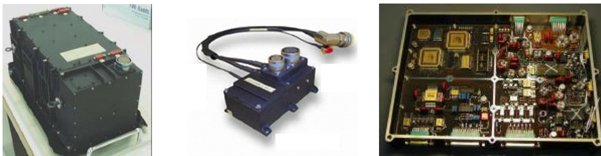
Figure 4. Flight model hardware: PPU, FU and PRE Card.
