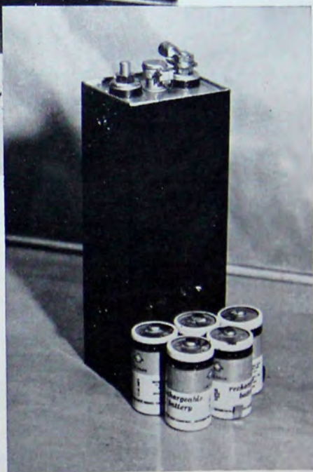
Fig. 10-A. A 1962-model of the original style Jungner Ni-Cd battery—five 30-ampere-hour cells to make a six-volt battery. Steel-cased cells are held and insulated in well-made hardwood racks. (Wood isn't new—but it's an excellent structural material still!) The steel cells must be insulated from each other. On the packing case lid beside the old-style Nicad are five sintered-plate cells—they yield six volts and four ampere-hours.
