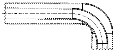
FIGURE B13.31 Example of an elbow whereby the inner elbow has a radius which is longer than that of the corresponding secondary containment elbow. (U.S. Patent 5,452,922; Orion Fittings, Inc.)
