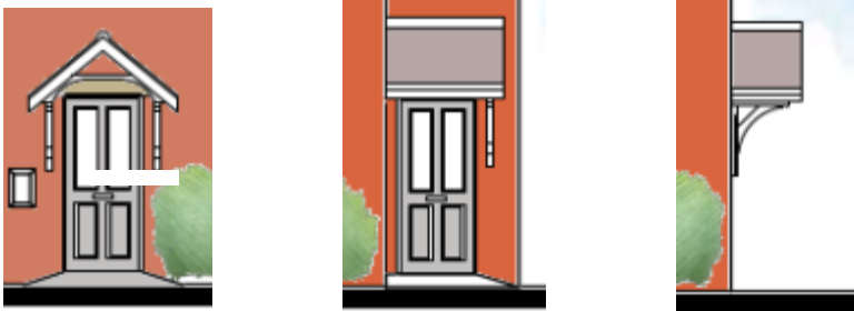
The use of varying canopy styles to front doors Typical of those used in the local area.
