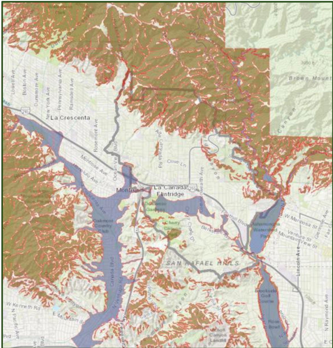
Figure 15: Landslide Zones in the City of La Cañada Flintridge
