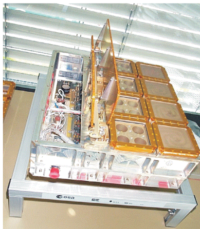
Fig. 1. External view of trays — equipment for exposing bacteria on the outside of the ISS
