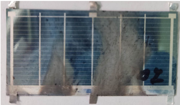
Fig. 4. Regolith particles deposited on the surface of the solar panel
