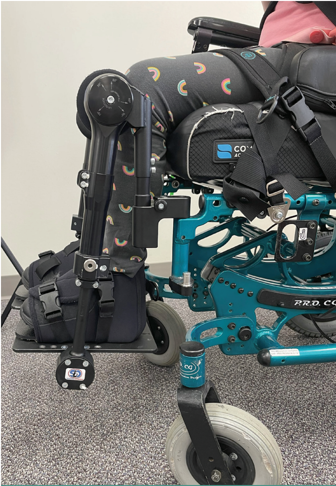
FIGURE 3 | The pivot point of the dynamic footrests (knee elevation feature) is close to the natural pivot point of the knee.
