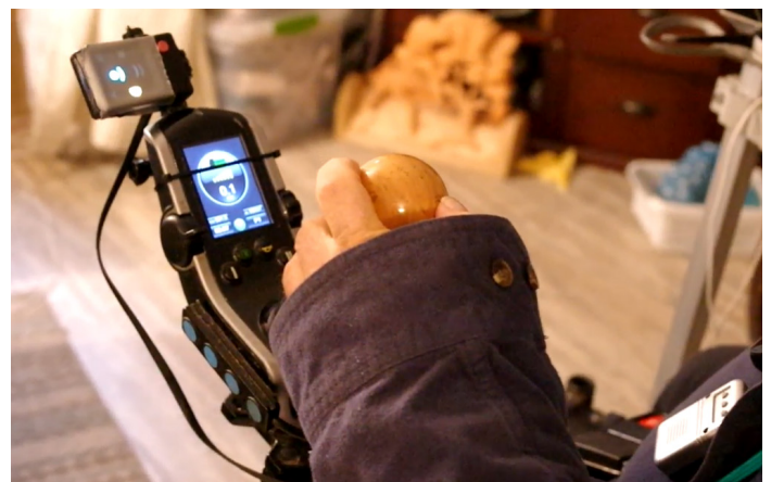
Braze Controller offering auditory and visual (LED) feedback from the Braze Blind Spot Sensors.
