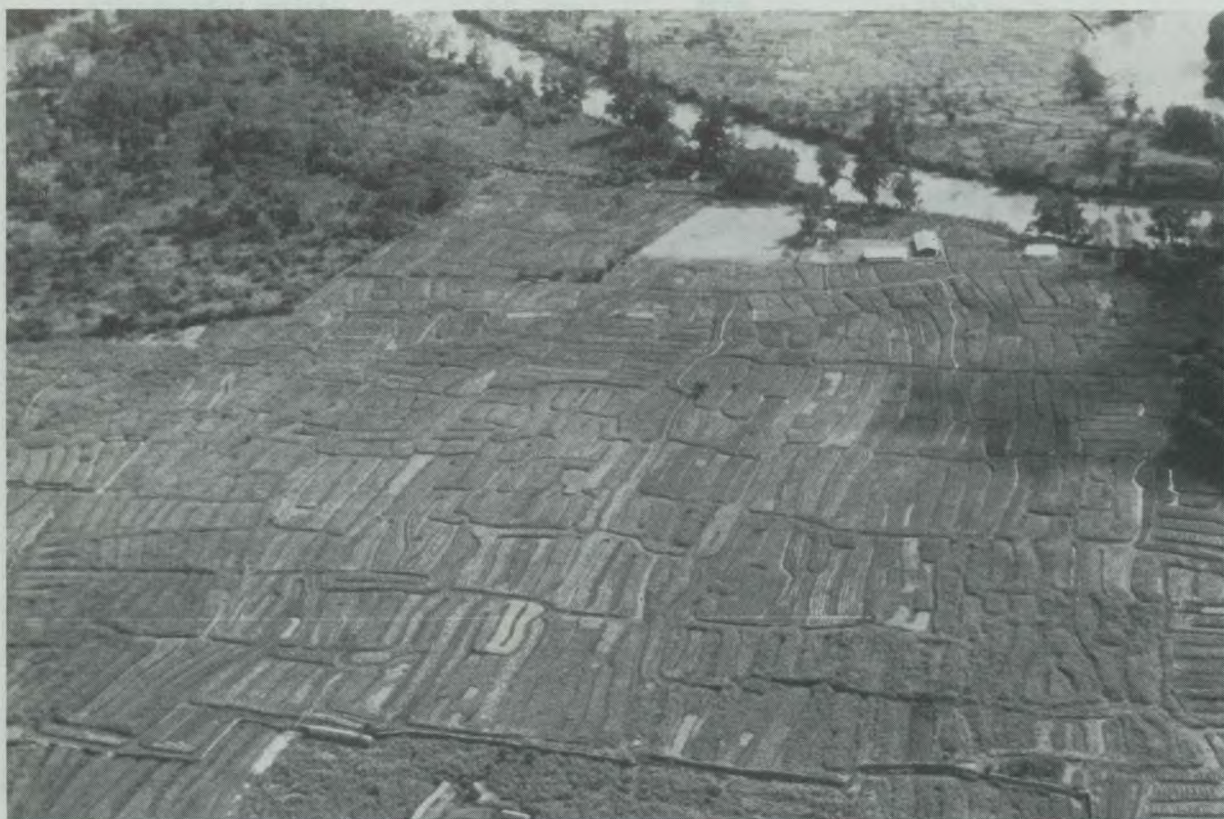
Plate 2 Aerial view of swamp drainage networks in the Baliem Valley, Irian Jaya. Canals may be up to hundreds of metres in length and be part of a field complex of up to 1.5 km 2 .
