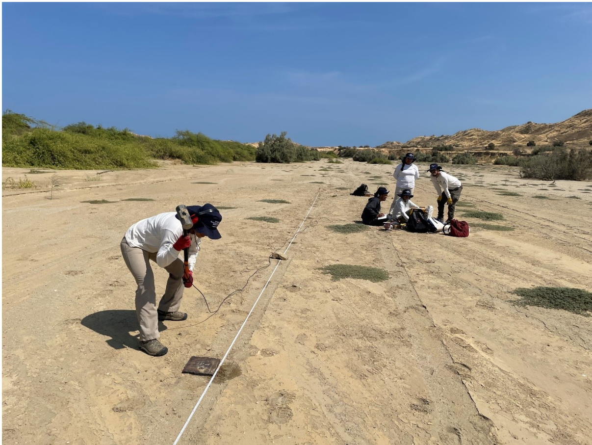
Fig 4. Seismic refraction survey layout and operation, Stage 1 (site 23090801).
