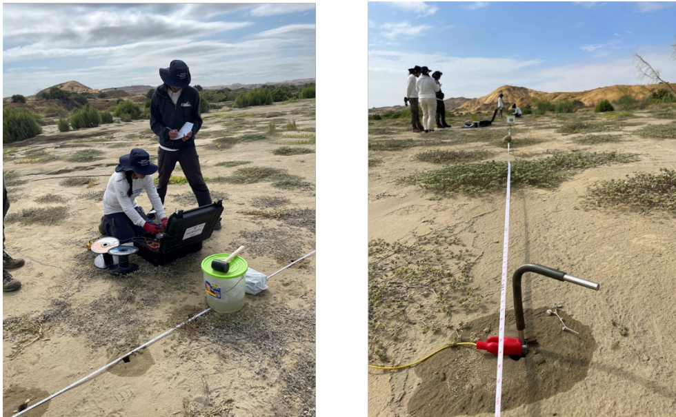
Fig 2. Photographs of the operation and layout of Stage 1 VES surveys in Quebrada Monte. Note the very dry surface conditions. High contact resistance due to the very dry surface soil was overcome by the addition of small quantities of nearby seawater to each electrode.
