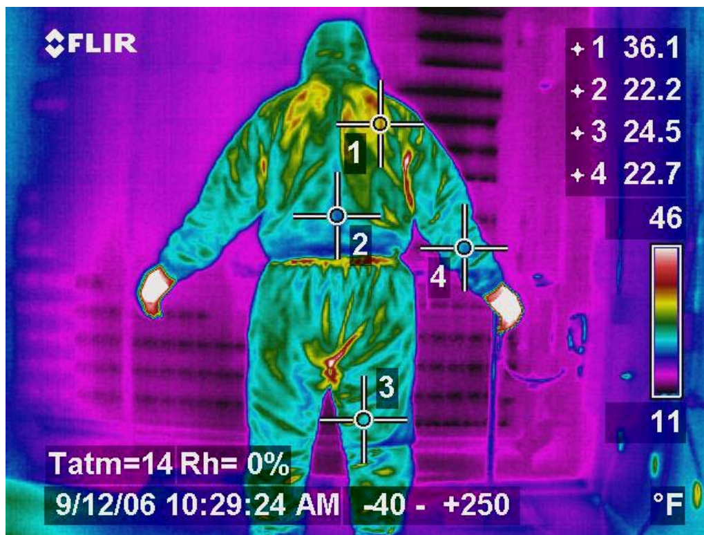
Figure 7. Back view of 400-weight Thinsulate garment (surface temperature range 22-36°F).
