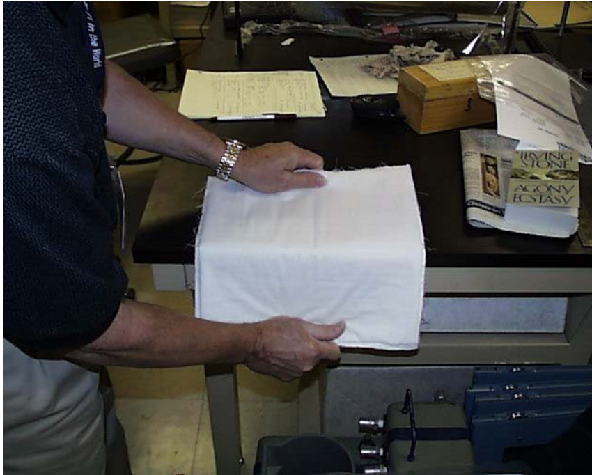
Figure 2. Sample of aerogel infiltrated, flexible fabric possessing ultra low thermal conductivity.
