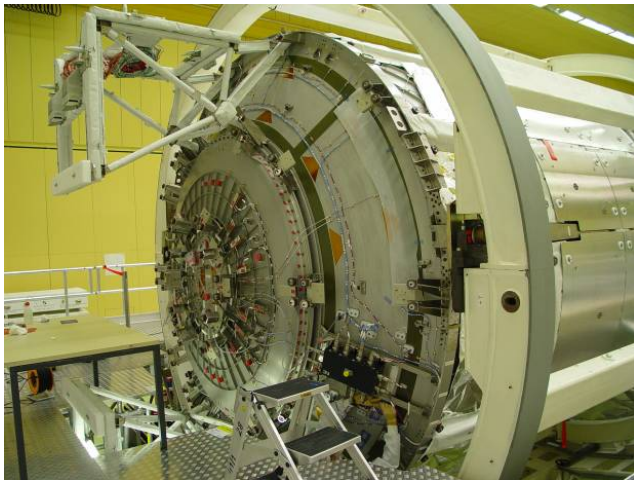
Columbus laboratory with External Payload Facility attached. August 2004
