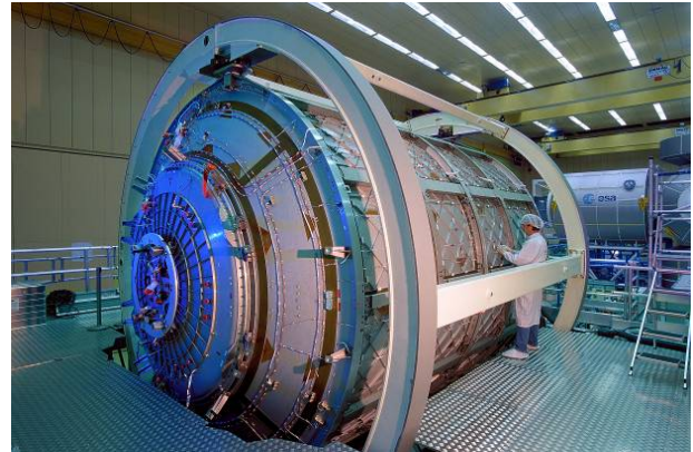
Columbus laboratory in Integration hall of EADS in Bremen. Primary structure exposed. June 2002
