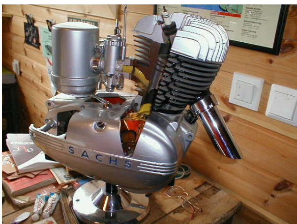
Picture 9 Cut-trough of a Sachs 175cc (Photo:Unknown)
