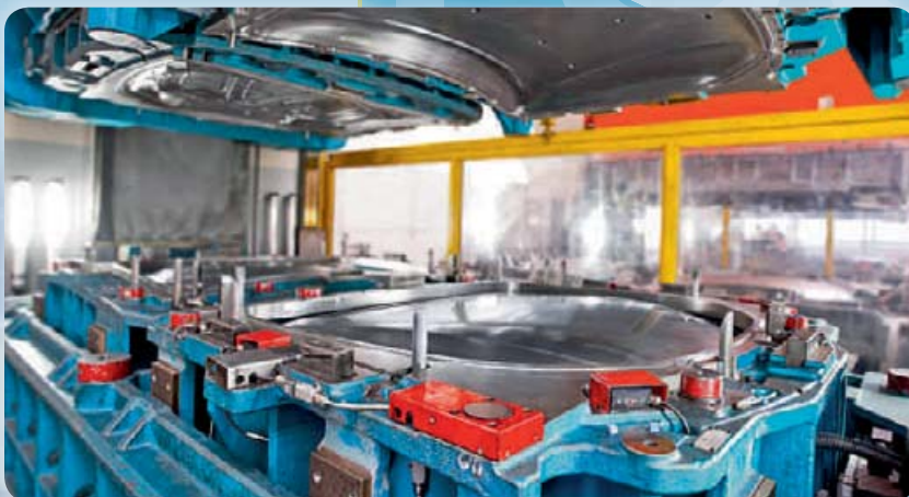
Perfection in toolmaking: A tool equipped with sensors is used to ensure optimal forming and efficient use of material.
