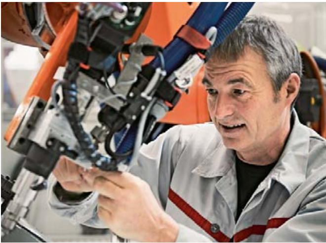
Industrial mechanic Peter-Michael Hahn inspects the filling valve on a gluing robot to ensure correct dosage.
