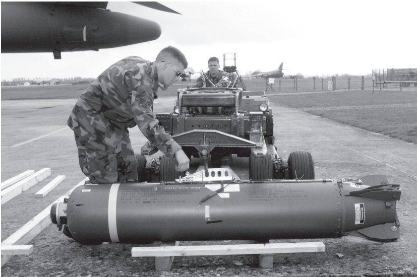
Deadly force. Munitions technicians at RAF Fairford prepare a CBU-87 cluster bomb unit for loading into a USAF B-1B bomber in preparation for a mission against fielded Serbian forces operating in Kosovo. With a loadout of 30 CBU-87s—more than five times the payload of an F-15E—the B-1 can fly at fighter-equivalent speeds more than 4,200 nautical miles unrefueled.
