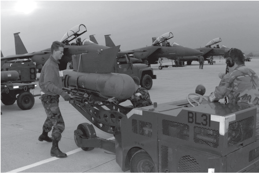
Eagle eye. Ground crewmen at RAF Lakenheath prepare a LANTIRN targeting pod to be mounted on an F-15E multirole, all-weather fighter. The pod, also carried by the Navy F-14D and the USAF F-16CG, contains a forward-looking infrared (FLIR) sensor for target identification at standoff ranges day or night, as well as a self-contained laser designator for enabling precision delivery of LGBs.
