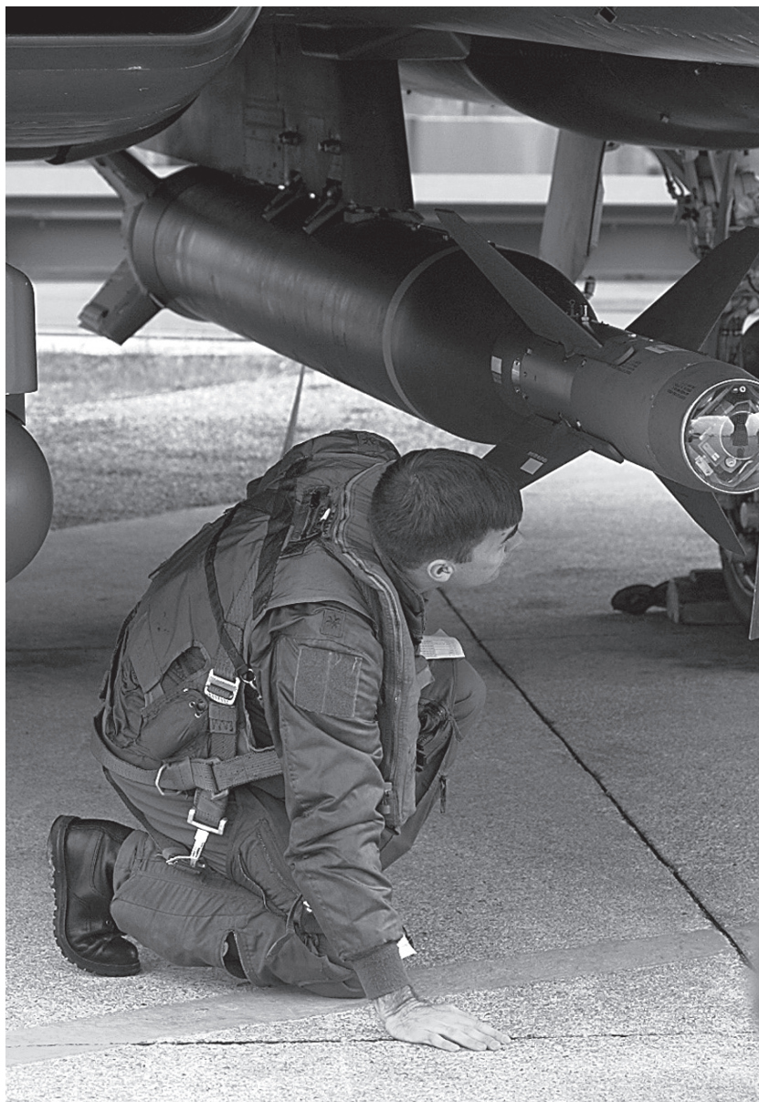
Hard-target killer. This F-15E pilot, a USAF major assigned to the 494th Fighter Squadron, looks over a 4,700-lb electro-optically-guided GBU-28 bunker-buster munition mounted on his aircraft's centerline stores station. The aircraft, one of a two-ship flight of F-15Es (call sign Lance 31 and 32), delivered the weapon on April 28, 1999, against an underground hangar at the Serb air base at Podgorica.
