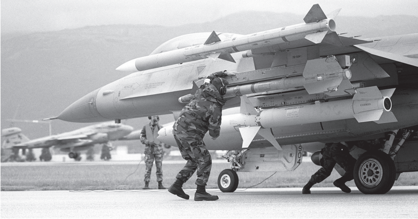
SAM hunter. This Block 50 F-16CJ in the arming area at Aviano shows an AGM-88 high-speed anti-radiation missile (HARM) mounted on the left intermediate wing weapons station, with an AIM-9M air-to-air missile on the outboard station and an AIM-120 AMRAAM on the wingtip missile rail. The USAF's F-16CJ inventory was stressed to the limit to meet the SEAD demand of Allied Force.
