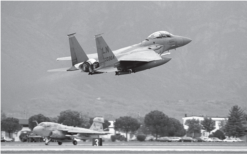
Burner takeoff. An F-15E from the 494th Fighter Squadron home-based at RAF Lakenheath, England, clears the runway at Aviano in full afterburner, with CBU-87 cluster munitions shown mounted on its aftmost semiconformal fuselage weapons stations. Eventually, some F-15E strike sorties into Serbia and Kosovo were flown nonstop to target and back directly from Lakenheath.
