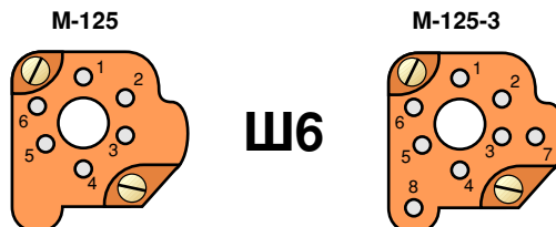
Pin-out of connector III6 of both the M-125 and the M-125-3
