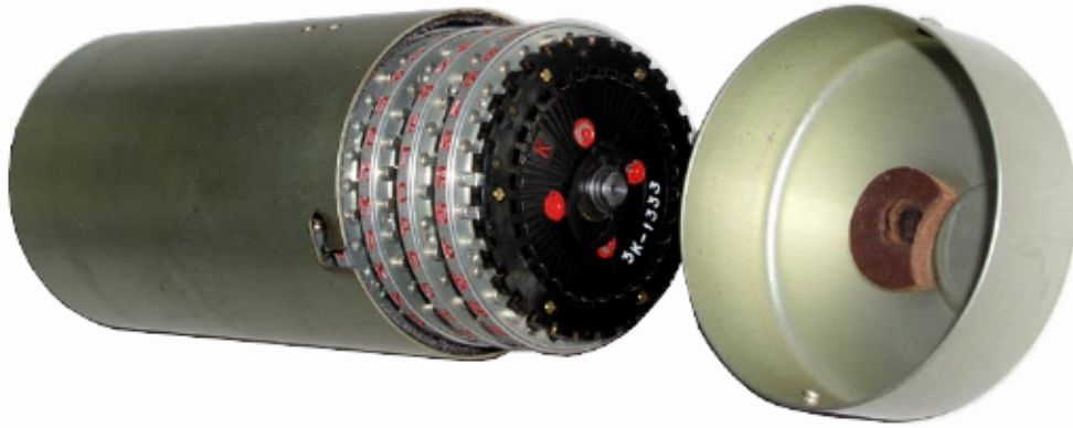
Spare wheel set in container. Photo by Tom Perera [4]
