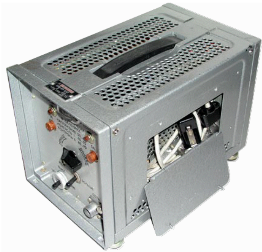
Power Supply Unit as supplied with Fialka machines in Poland. Photo by Tom Perera [4]
