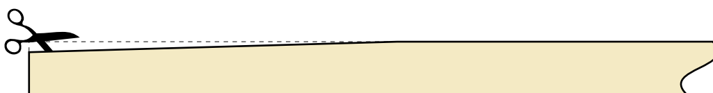
Modifying the 10 mm tape for easy insertion
