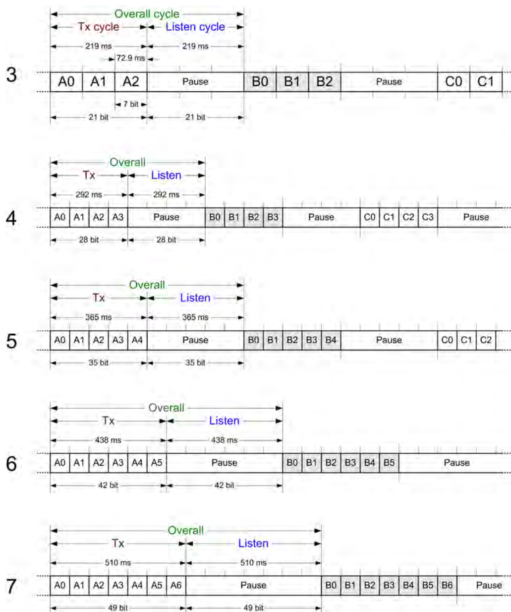
Fig. 3-21: Timing of an ARQ-S cycle at 96 Bd baud rate.
