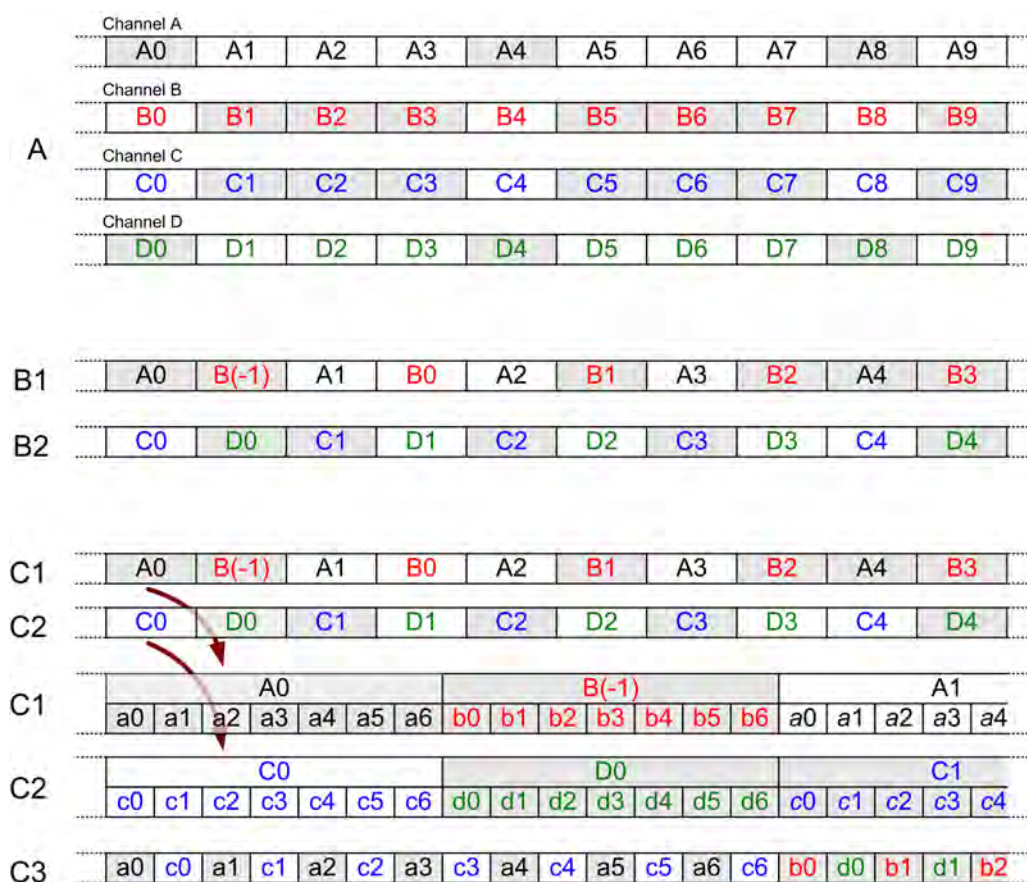
Fig. 3-20: Interleaving scheme for ARQ-Mx-342 (4-character repetition cycle).
