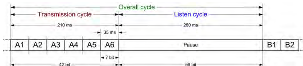
Fig. 3-17: Timing of an ARQ 6-98 cycle.
